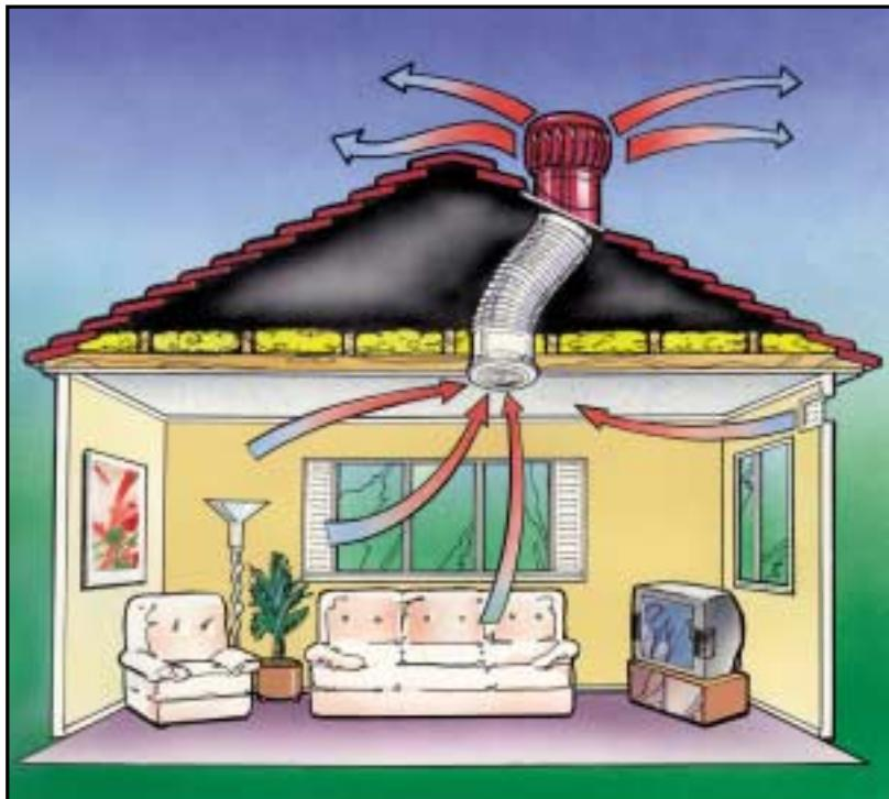
The **Bathroom Vent System** is designed for the continuous extraction of moisture and odours from bathrooms. It incorporated the 150mm Turbo Ventura ventilator, 3m of ducting and a controllable 150mm round ceiling register.
